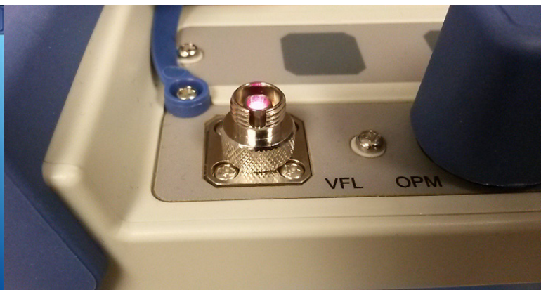
Pictured: Visual Fault Locator (VFL) beam illuminates bends, splices, and faults in optical fibers, with an effective range of up to 10km.
