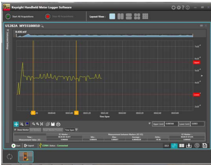
Figure 2. U1282A data log trend plot with markers and limit levels.
